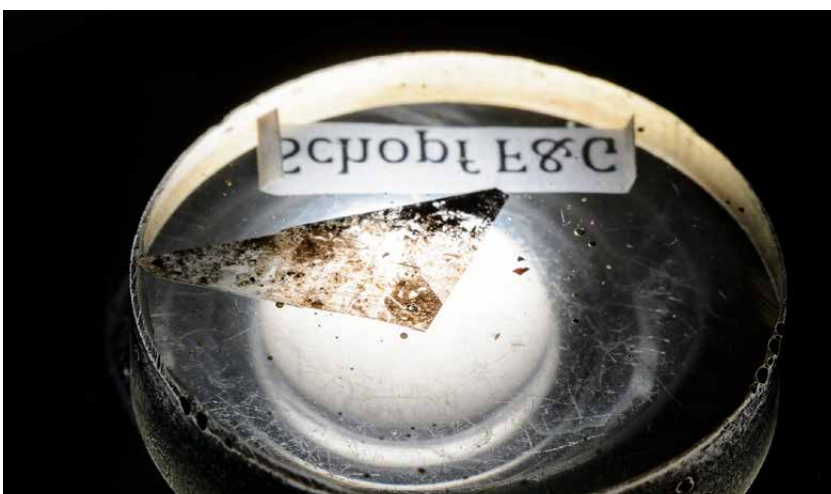
An epoxy mount containing a sliver of a nearly 3.5 billion-year-old rock from the Apex chert deposit in Western Australia is pictured at the Wisconsin Secondary Ion Mass Spectrometer Lab in Weeks Hall. Jeff Miller
