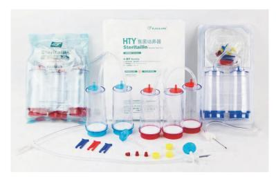
The complete sterility test system includes the Sterility test pump and sterility test kit. It is a closed system to avoid the extraneous contamination. Steriltalin® sterility test kits provides many kinds of test kits to fit for variety of drugs and packages.
